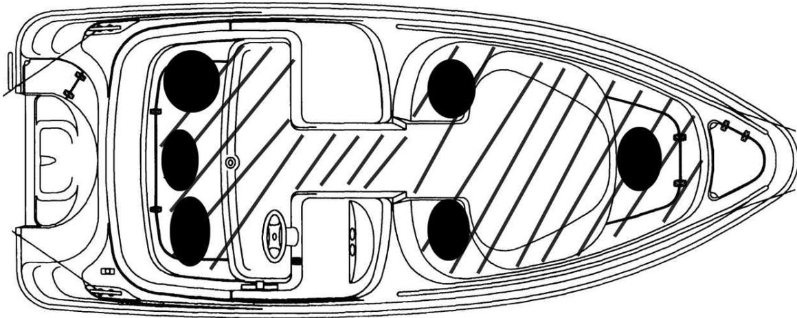
YAMARIN 50 Side Console/ YAMARIN 50 S Side Console      Seats for the maximum recommended number of persons and working decks
